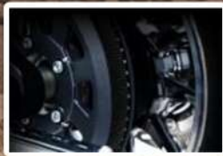
Gate Belt Transmission
