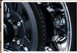
Gate Belt Transmission
